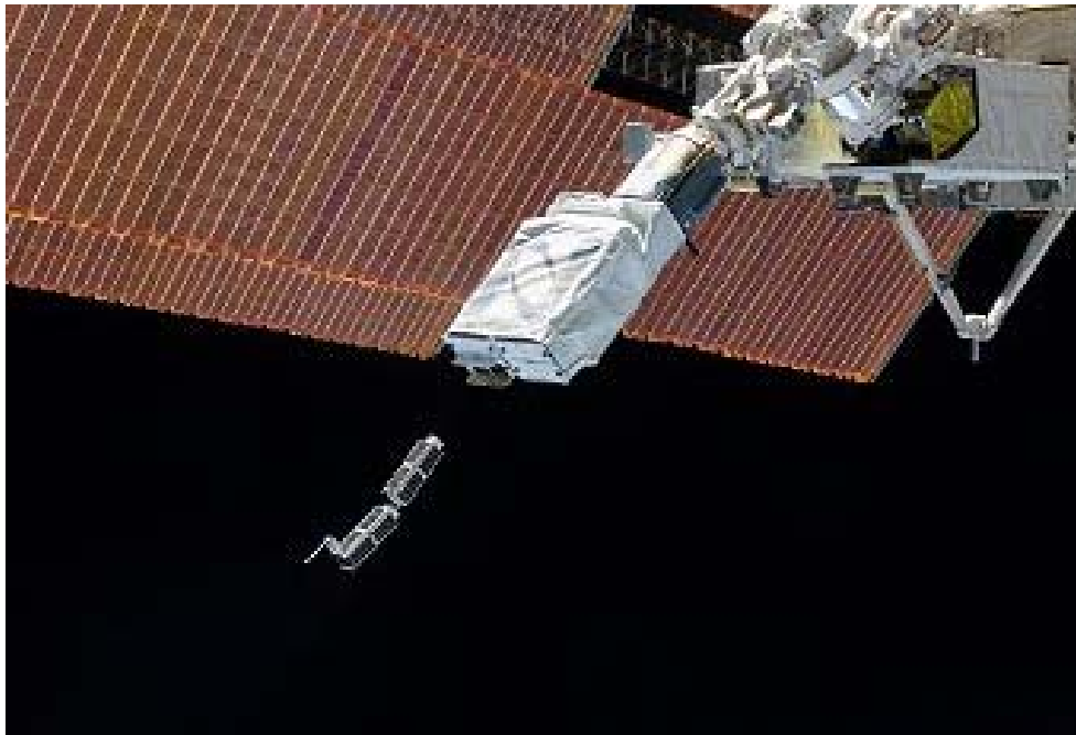
Figure 4-2 NanoRacks CubeSat Deployer
